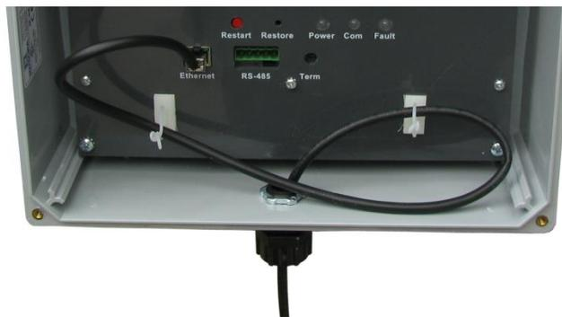
Figure 10: Ethernet cable routing and connection
