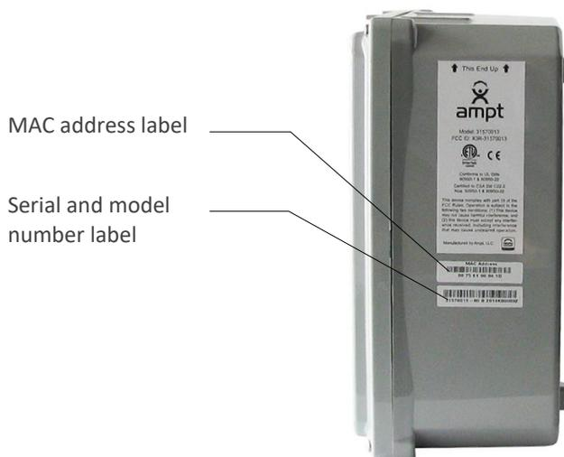
Figure 3: Serial number, model number, and MAC address labels
