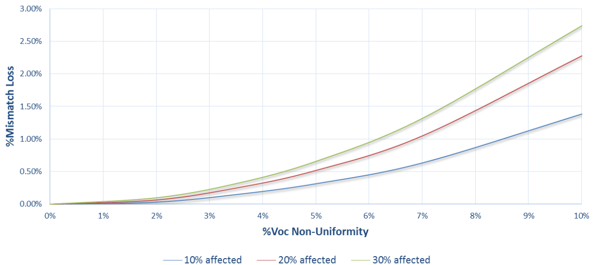
7 %Mismatch Loss due to non-uniformity in voltage by varying amounts of the array affected.
